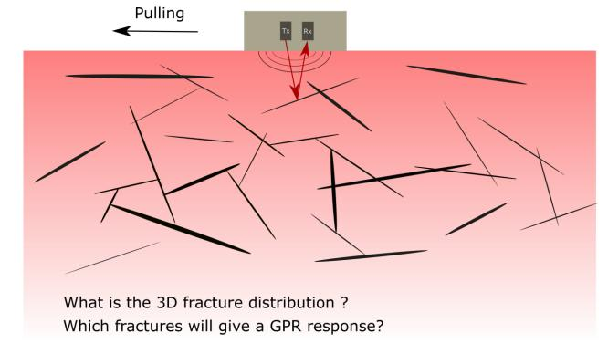
The first field campaign aimed at imaging the 3D distribution of the main open fractures using surface GPR. Our experiments were acquired in a tunnel of dimensions 22 x 3.6 x 4.8 m located at 410 m of depth. Since the floor was sawed, the conditions to acquire surface GPR were ideal. The tunnel geology is composed of granite, diorite and granodiorite [Ericsson et al. 2015].
