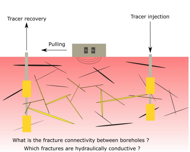
To infer fracture connectivity patterns, we conducted surface GPR during tracer test injections. Because of the saline formation water (≈1850 mS/m), we injected deionized water to achieve an electrical contrast. At the same time, we used traditional Uranine and Rhodamine tracers.
