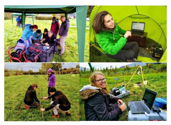
Photos: From top left, clockwise: Borehole SIP, seismic refraction, borehole GPR, ERT. Credits F. Nguyen
