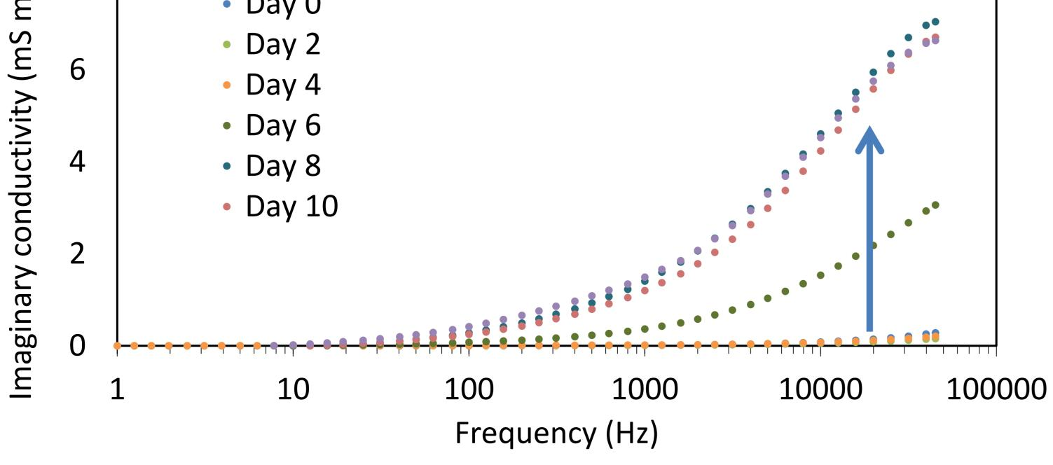
Imaginary conductivity increased due to calcite precipitation.
